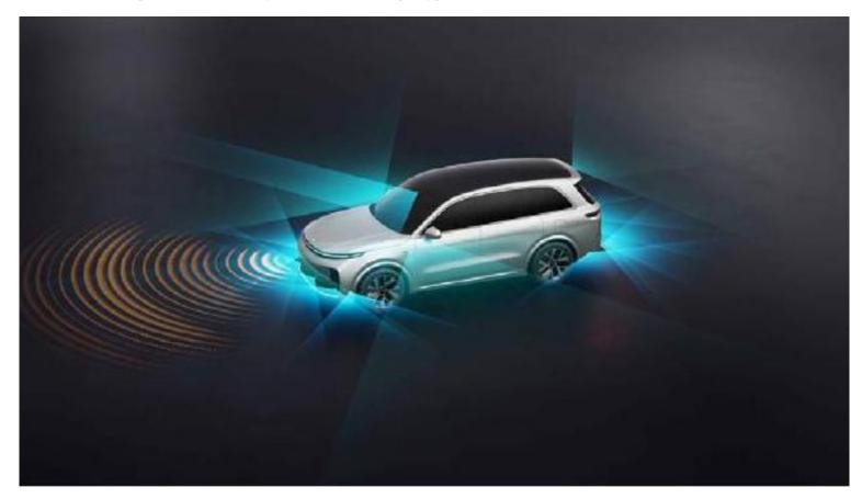
Li L8 Max comes standard with Li AD Max autonomous driving system, powered by dual Orin-X chips with 508 TOPS of computing power, enabling real-time, efficient processing of fusion signals from high-definition cameras, LiDAR, millimeter wave radar, and ultrasonic sensors. The dual processors provide fallback redundancies for each other, ensuring a more stable operation of the autonomous driving system.
